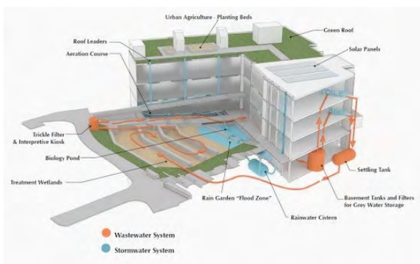
Figure 8. The pond and rain garden prevent storm water runoff. Source: http://www.sidwell.edu/middle_school/ms-green-building/index.aspx
