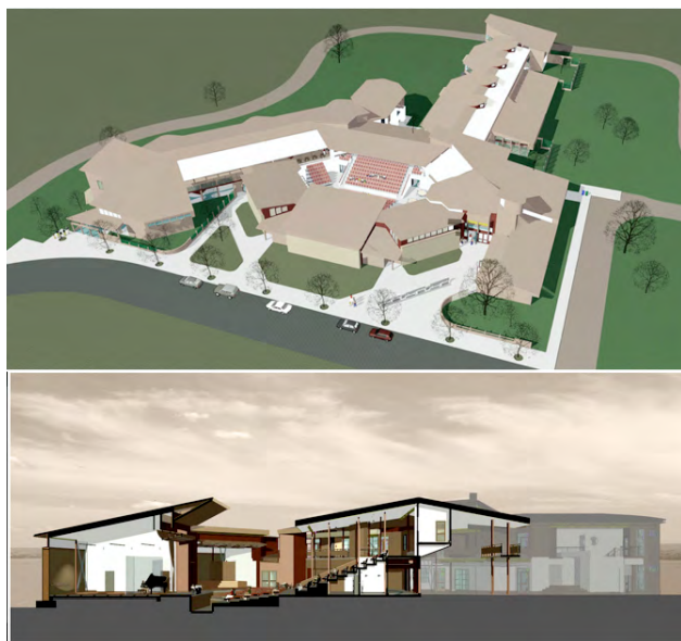
Figure 23. 3D model and section illustrate the design of the school and central outdoor theatre. Source: Arts, 2011.
