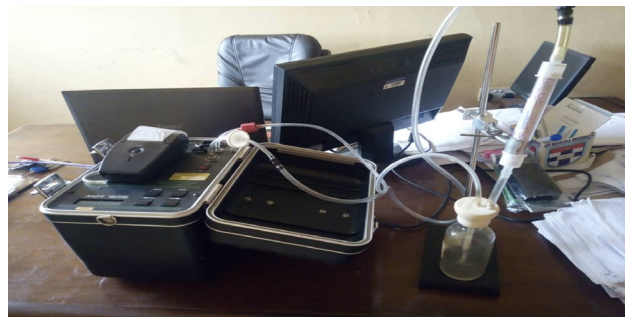
Figure 2. The RAD-7 experimental set-up for radon in water measurement.
