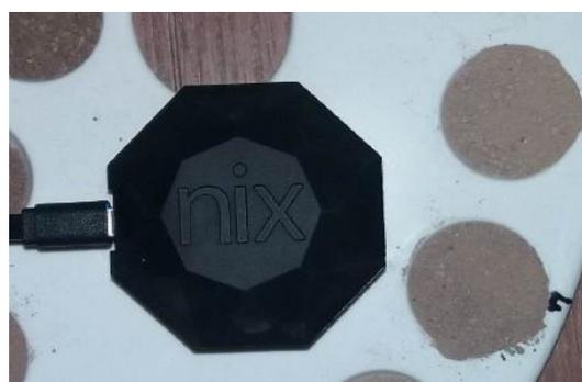
**Figure 3.** The Nix Pro™ sensor connected to a smartphone and soil samples sieved at 0.5 mm.
