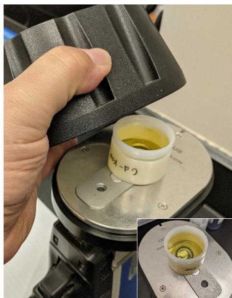
**Figure 1.** Experimental configuration using a Field Stand-V to mount samples. Pictured here are liquid samples containing Cd, placed directly over the portable X-ray fluorescence (PXRF) spectrometer aperture, and scanned in sample cups featuring Kapton thin film.
