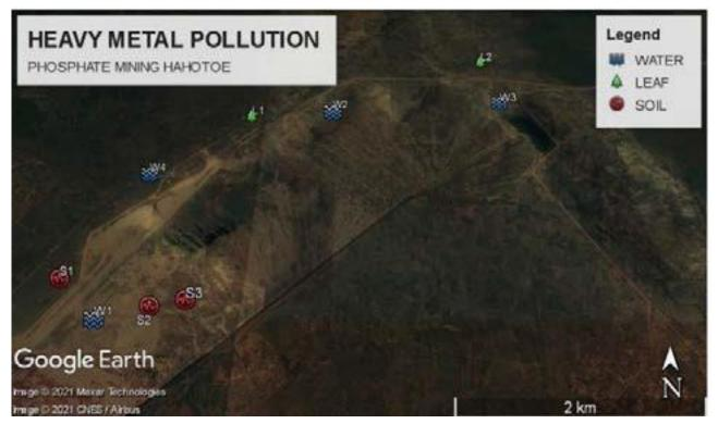
Figure 2. Google Earth map of the Kpémé phosphate processing area showing the different samples collected
