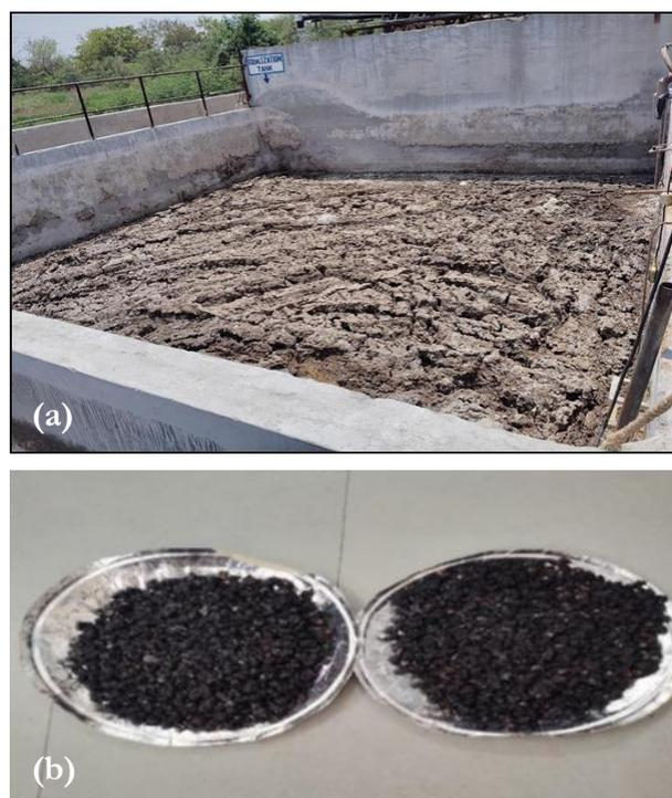
**Figure 1.** (a) Dairy processing sludge tank at Saras Dairy Plant, Kota; (b) Biochar produced from DPS
