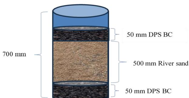
Figure 2. Schematic diagram of filter media
