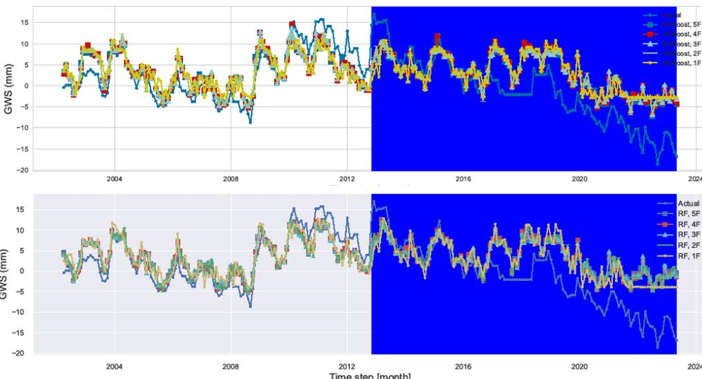
Figure 9 Comparison of mean actual and XGBoost predicted groundwater storage (GWS) over the region of interest for different selected features, all curves in one plot.
