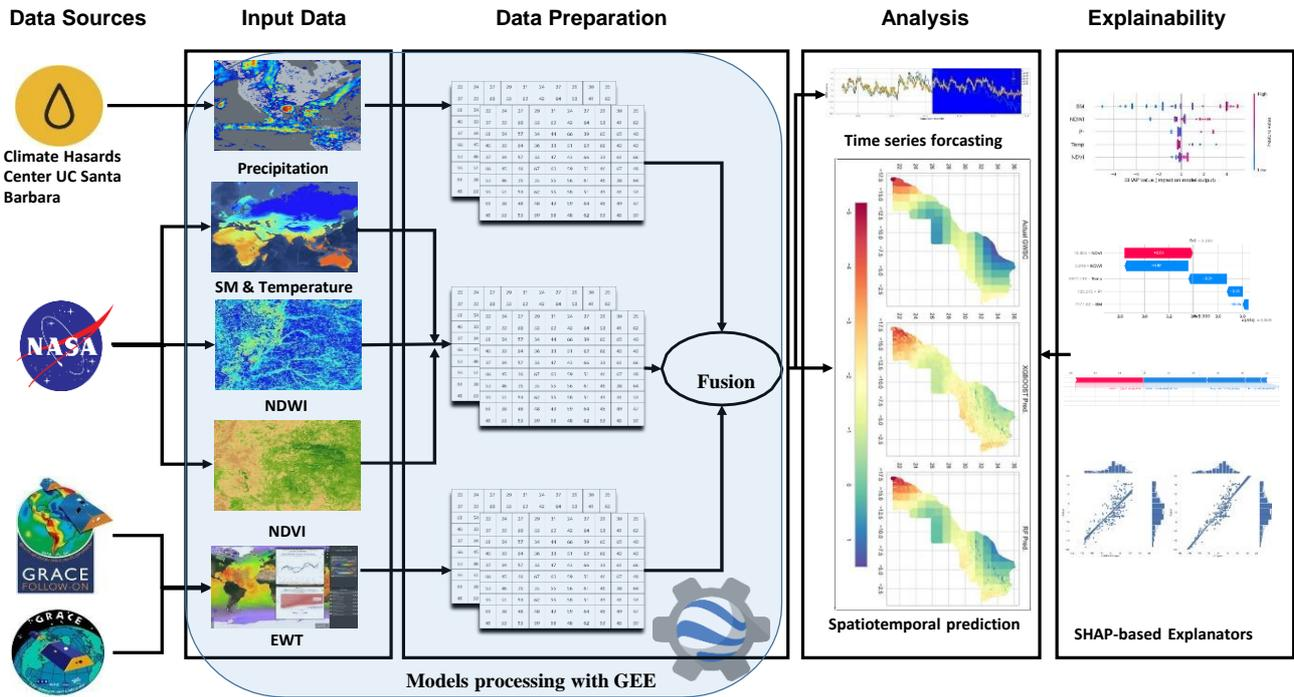
Figure 3. Groundwater storage management workflow using artificial intelligence and remote sensing adapted to the data science process.
