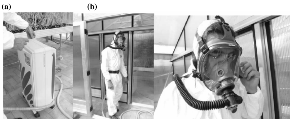
Figure 1 - Special care was taken to protect the operators who worked in part B of the greenhouse: (a) electrofilter; (b) facial mask with external air supplier
