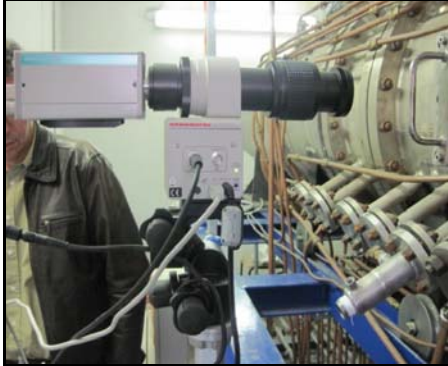
Figure 16 - LIF image intensifier and CCD camera
