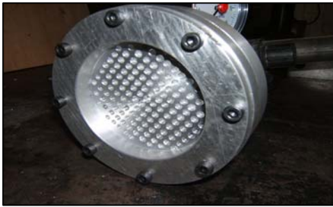
Figure 9 – Inner disk holding the multi-membrane arrangement
