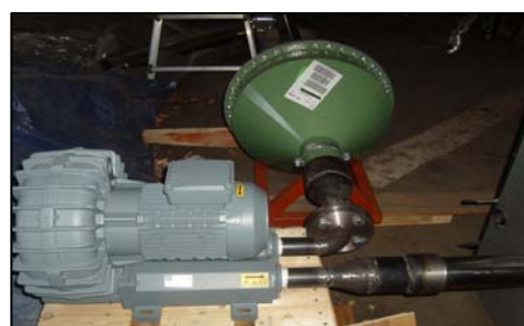
Figure 12 – The filter connected to the blower
