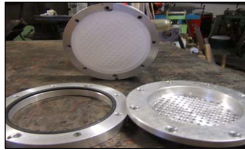
Figure 10 – Multi-membrane filter nearing completion
