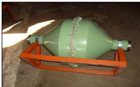
Figure 11 – Multi-membrane filter mounted on its trestle
