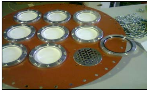
Figure 11 – Multi-membrane filter mounted on its trestle
