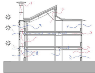
Figure 8b. Environmental response and smart spaces, The Building Research Establishment (BRE) Office Building, shows the solar chimneys and details of the solar station as well as solar fenders moving aesthetic dimension (DeKay and Brown, 2001).
